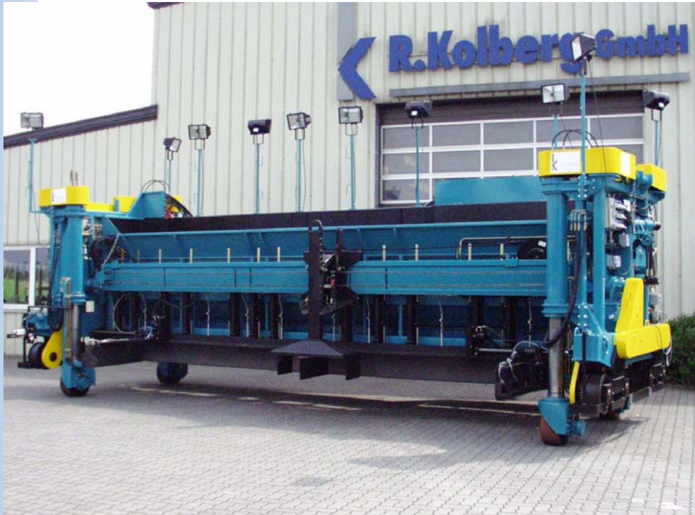
Gussasphalt (mastic asphalt) – finisher KBR 75 on extended hydraulic pillar ready to load on low platform trailer
