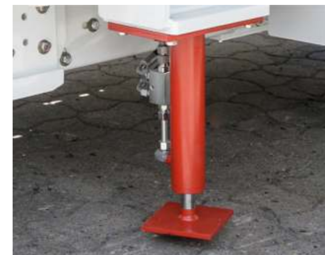
Hydraulic foot for variable height adjustment.
