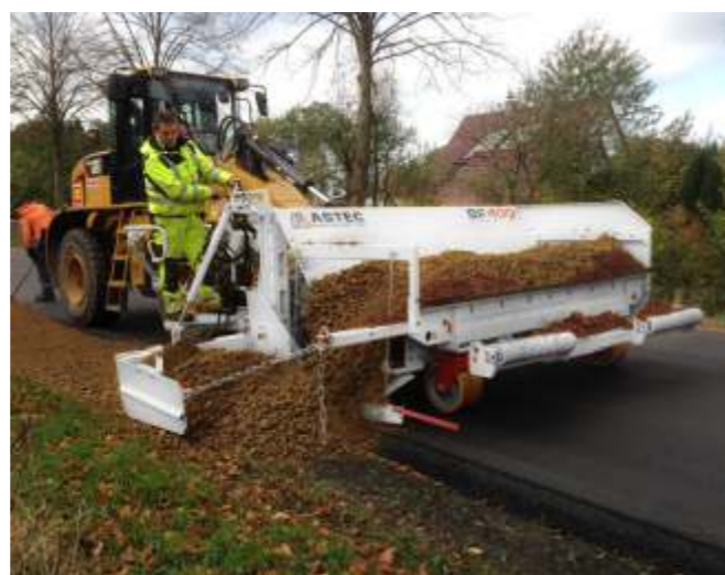
big hopper carries 4,0to of material - easy operation, fast and economical
