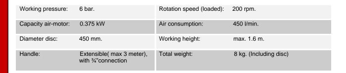
Discs with diameter 450 mm including nylon screws are available separate.
